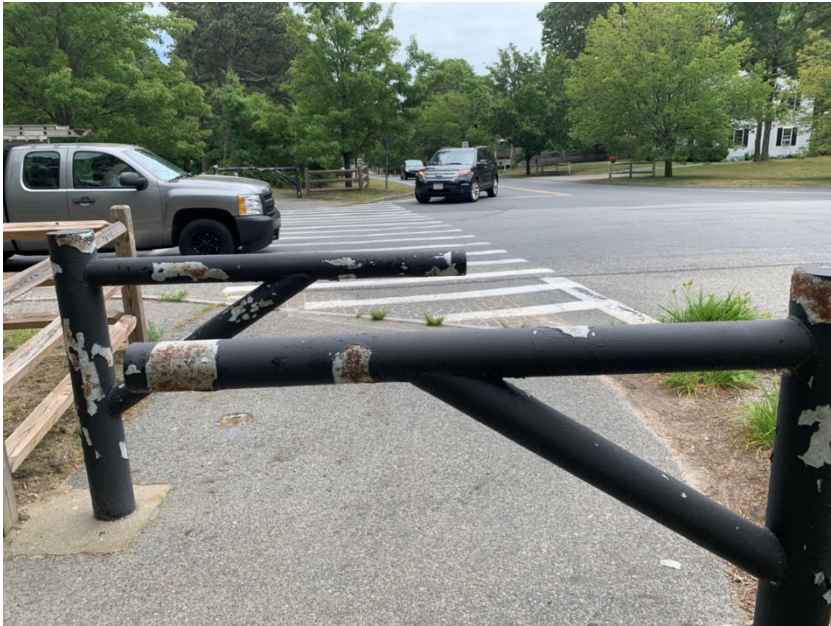
Figure 208: Barriers Require Bicyclists to Slow/ Walk Across Before Crossing. Continental Crosswalk Improved Visibility.
